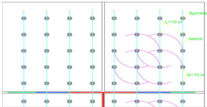
**Figure 3.** layout of fixed sprinkler system network
