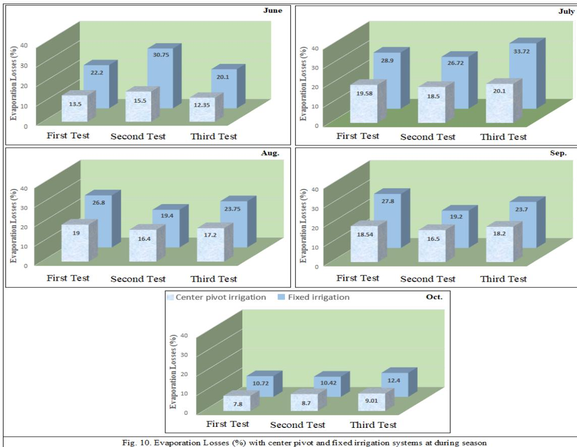
Fig. 10. Evaporation Losses (%) with center pivot and fixed irrigation systems at during season
