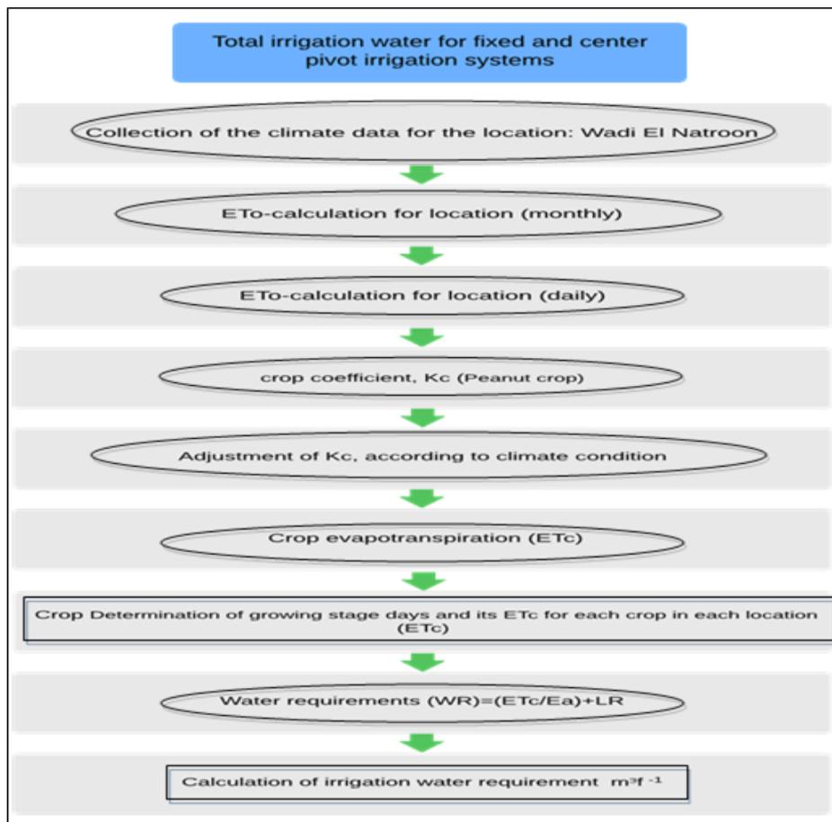
**Figure 4.** Process planned of method for calculating the irrigation requirements of peanut crop
