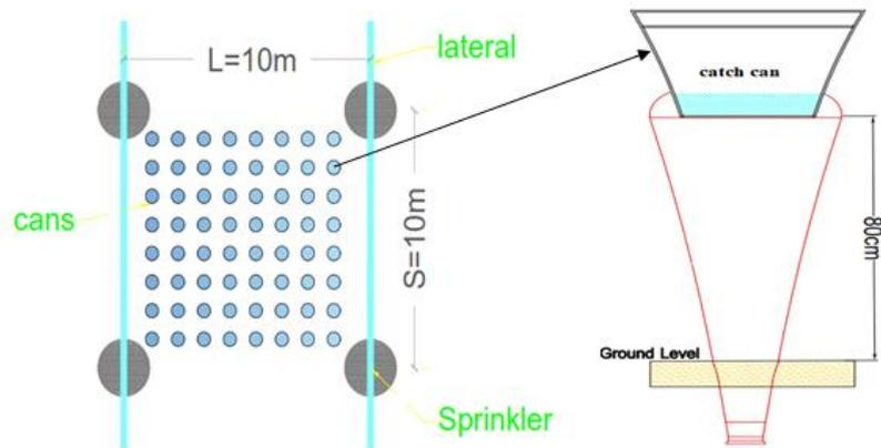
**Figure 5. Layout the sprinklers in the field to test the uniformity for fixed irrigation system**
