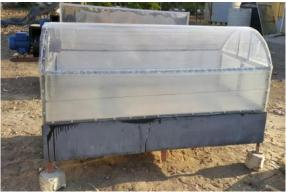
Fig. 1b. Modified-Quonset solar dryer
