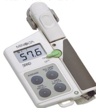
Fig. 2. Portable chlorophyll meter SPAD-502 for measuring relative chlorophyll content
