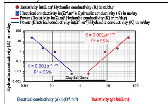
Fig. 14. The relation between Average true resistivity or electrical conductivity and typical hydraulic conductivity values of the recorded soils.
