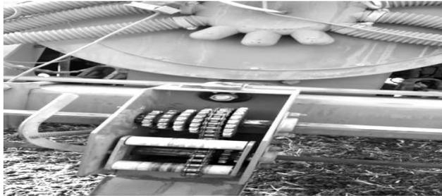
Fig. 7: Gear box for change grain plate speeds.
