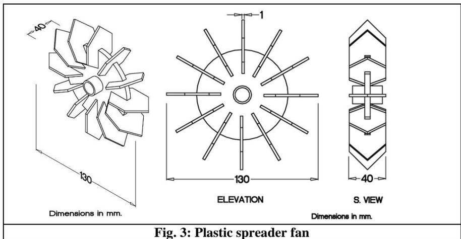
**Fig. 3: Plastic spreader fan**
