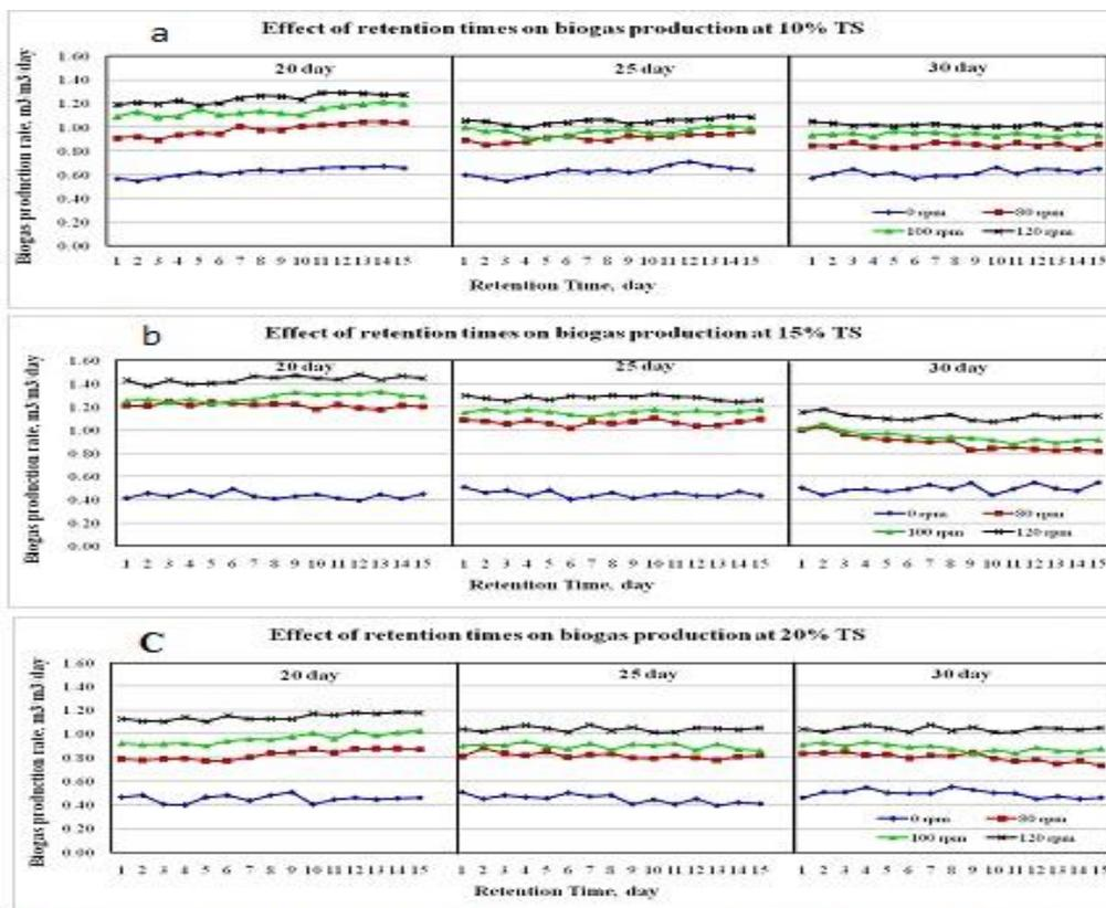
**Figs. (6a, b and c) The effect of retention time on Biogas production rate (m<sup>3</sup> / m<sup>3</sup>/day) at 20, 25 and 30 day retention time after steady state phase**
