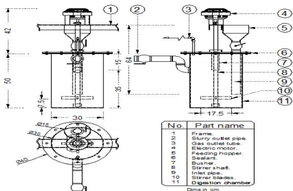
Figure 1a. Elevation, side view and plan of one digester
