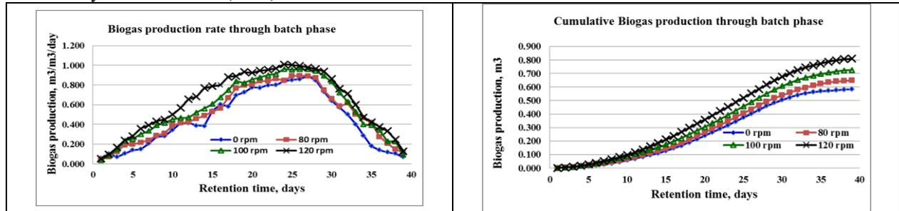
**Fig. 3a. Biogas production rate  $\text{m}^3/\text{m}^3/\text{day}$  through batch phase**
