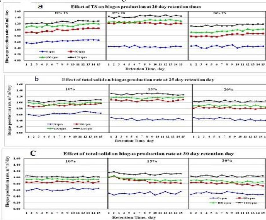
**Figs. (5a, b and c) The effect of total solids concentration on Biogas production rate ( $\text{m}^3/\text{m}^3/\text{day}$ ) at 25 and 30 day retention time after steady state phase**
