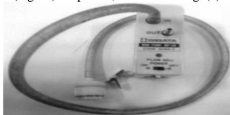
**Fig. 6. The personal dust sampler.**
