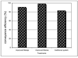
Fig. 11. Conveyance efficiency (%) with all treatments
