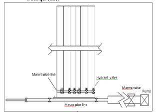
Fig. 4. Layout of the irrigation system developer by Marwa (s<sub>3</sub>).
