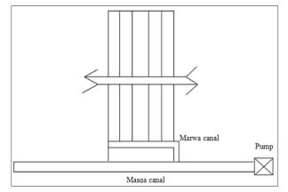
Fig. 2. Layout of the traditional irrigation system  $(s_1)$ .
