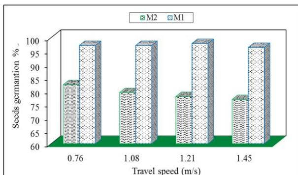
Fig. 9. Effect of travel speed (m/s) and sowing modes on seeds germination %.
