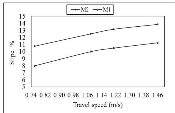
Fig. 7. Effect of travel speed (m/s) and sowing modes on slip %.
