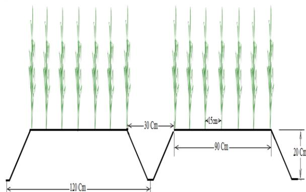
**Fig. 3. Sketch of the proper raised-bed.**
