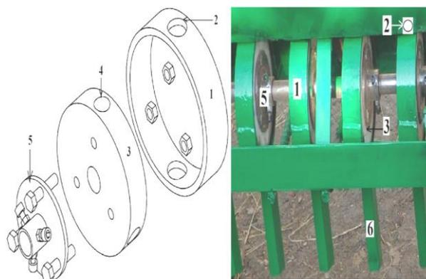
**Fig. 4. The seed metering mechanism.**
