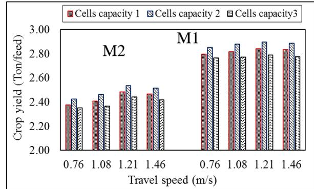
Fig. 10. Effect of travel speed (m/s), two sowing modes and disc cells capacity on crop yield (ton/fed).
