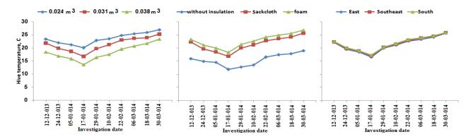
Fig. 5: Effect of the internal hive size, insulator type and hive entrance direction on hive temperature, °C
