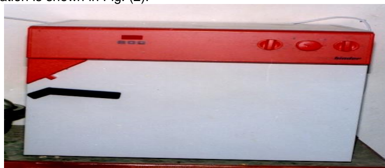
Fig.(2):The electrical oven used for determination of grain moisture content.
