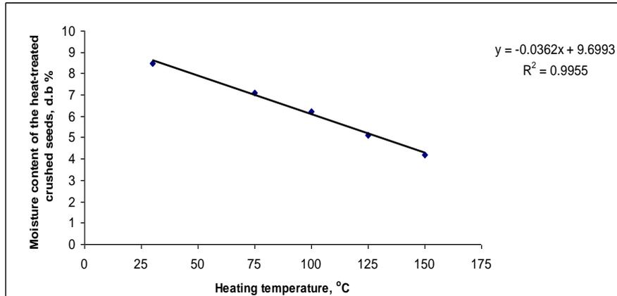
**Fig. (3): Moisture content of crushed seeds as a function of heating temperature.**
