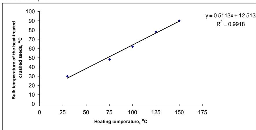
Fig. (2): Relationship between bulk temperature and heating temperature
