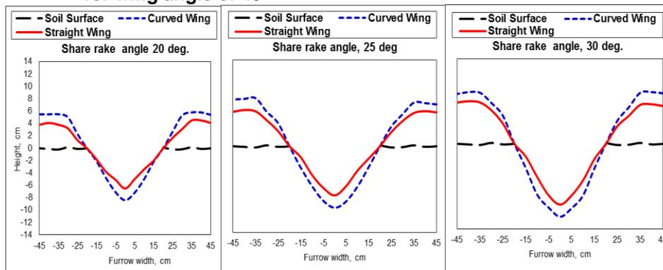
**Fig. 5: Furrow profile as influenced by share rake angle and wing shape for wing angle of  $35^\circ$**
