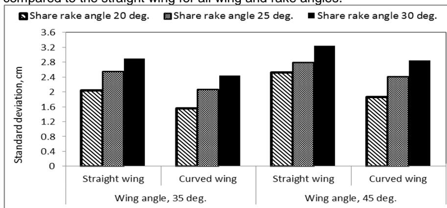
**Fig.5: Effect of share rake angle, wing angle and wing shape on standard deviation of seeds scattering, cm**
