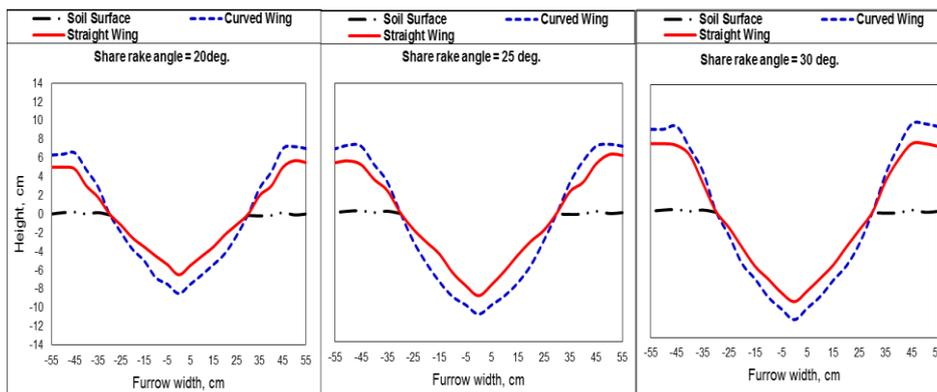
**Fig. 4: Furrow profile as influenced by share rake angle and wing shape for wing angle of  $45^\circ$**
