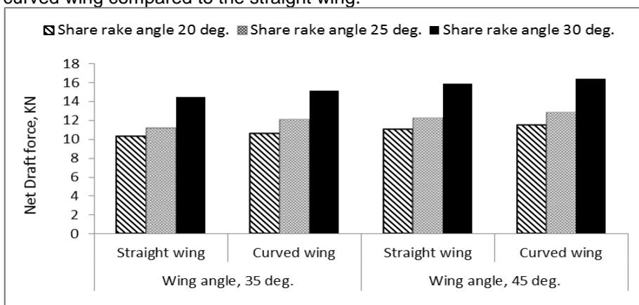
Fig. 6: Effect of share rake angle, wing angle and wing shape on net draft force, kN.
