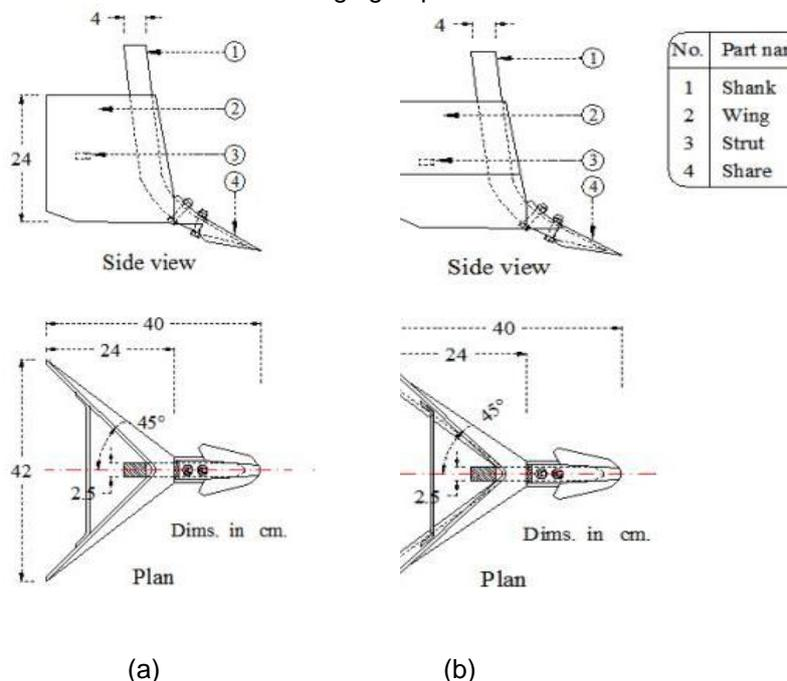
**Fig. 1: Straight opener wing (a) and curved wing (b)**
