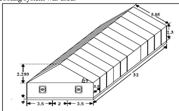
Fig. 1. Commercial gable-even-span greenhouse (dimensions in metre).
