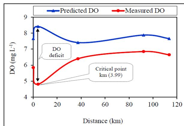
**Fig. 2. Predicted and measured DO sag curve of studied River for August.**
