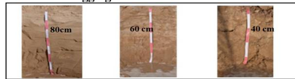
Fig. 8. The water table level at different locations on the “AB” transect.
