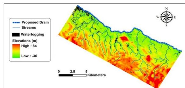
Fig 10. A suggested surface drainage network.
