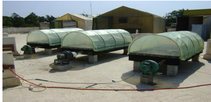
Fig. (1): Solar tunnel greenhouses (Quonset type) used as an active solar dryers during the experimental period.
