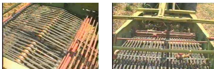
Fig (4): Front elevator and ray separator and vibrator after development
