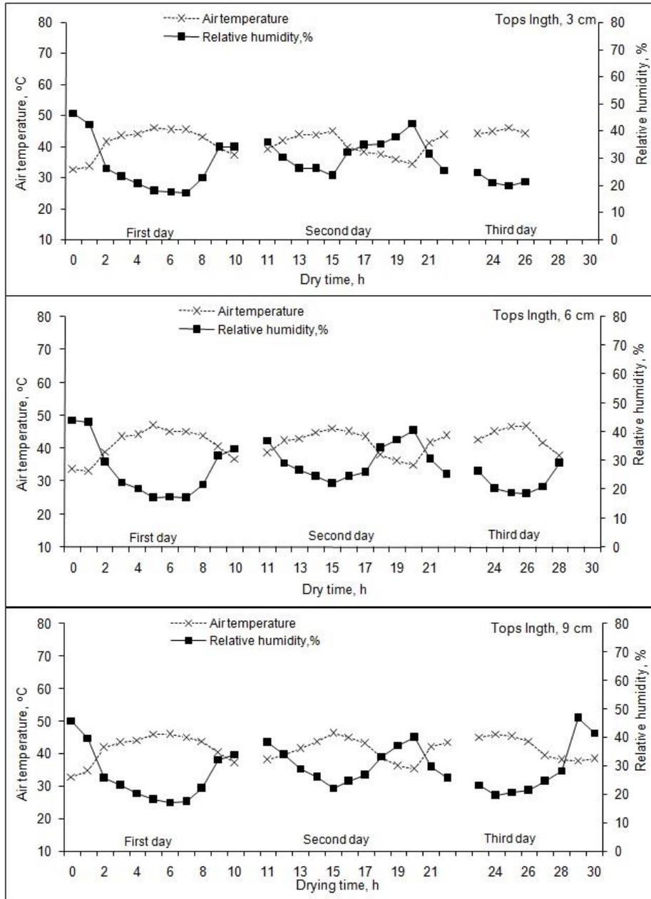
Fig. (6): Air temperature and relative humidity as related to drying time using the minimum air velocity of 0.4 m/sec (chopped green tops).
