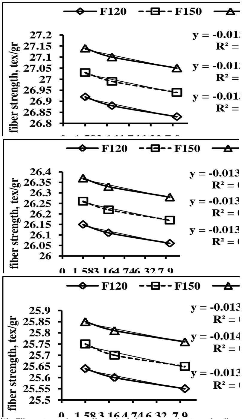
Fig. (6): Fiber strength as affected of drum speed, straw feeding rate and straw moisture content.
