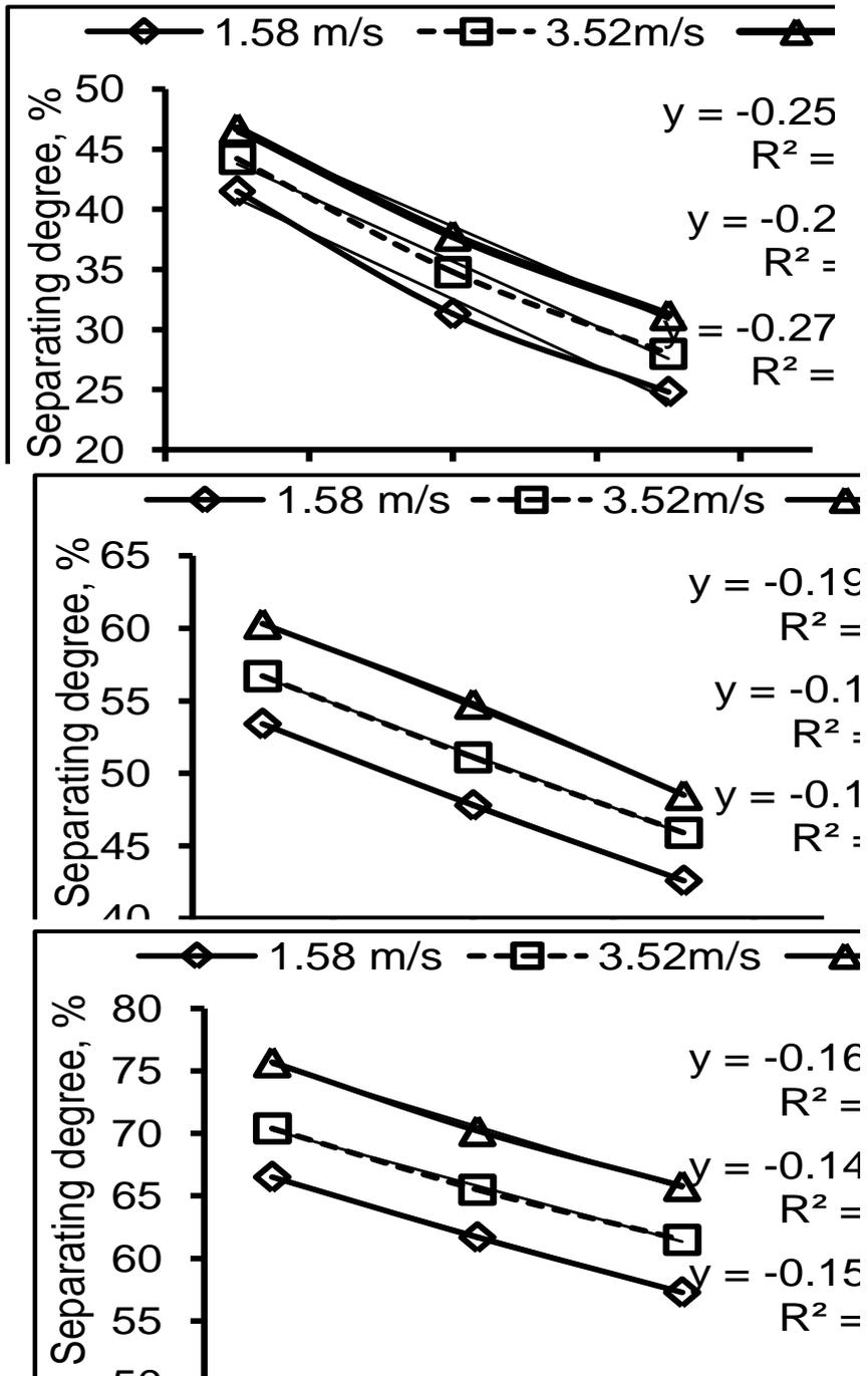
Fig. (4): The separating degree (%) of flax fibers as affected by straw feeding rate.
