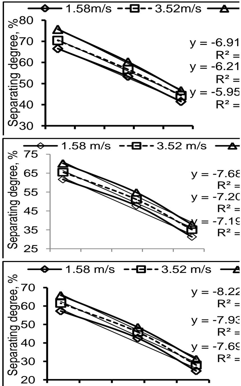
Fig. (5): The separating degree (%) of flax fibers as affected by straw moisture content
