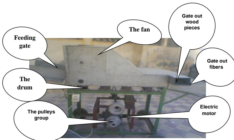
Fig. (1): The sketch of the developed machine for separation flax fiber
