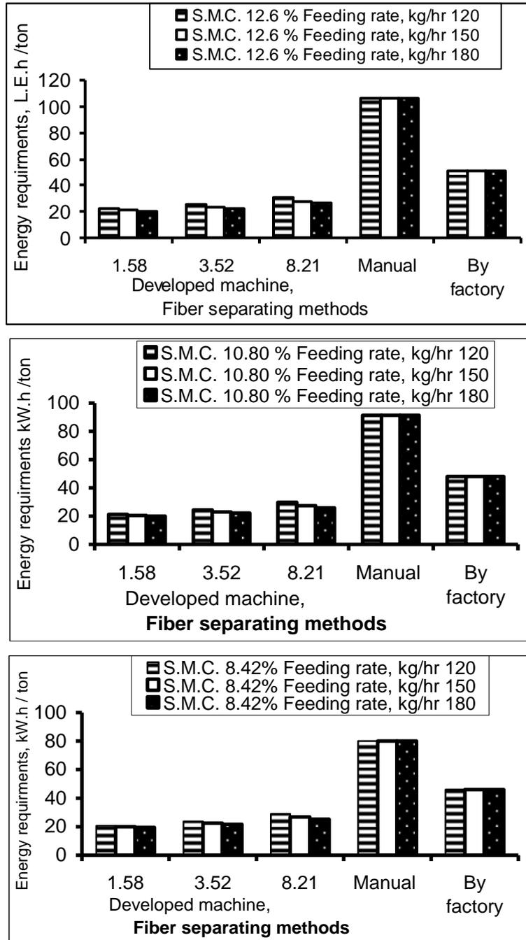
Fig. (6): Energy requirement (kW.h/ton) for separating methods under different drum speed, feeding rate and straw moisture content.
