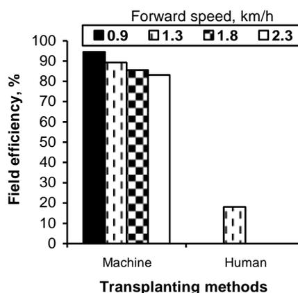
**Fig. 8: Effect of transplanting methods on field efficiency.**
