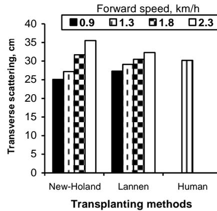
**Fig. 4: Effect of transplanting methods on transverse scattering.**
