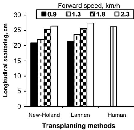
**Fig. 3: Effect of transplanting methods on longitudinal scattering.**
