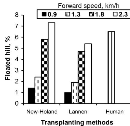
**Fig. 6: Effect of transplanting methods on floated hill.**
